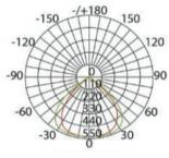
UNIT:CD/KLM -C0/180,88.2deg C90/270,98.2deg AVERAGE BEAM ANGLE (50%):93.2 DEG
